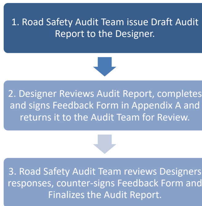
Figure 4.1 – Road Safety Audit Sign-Off and Completion Process
